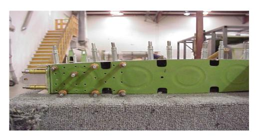
7/ Bolt the hinge brackets back on first to allow maximum space for wrenches, then rivet the doubler on, then rivet skin back on to the rib. Repeat for other side.
