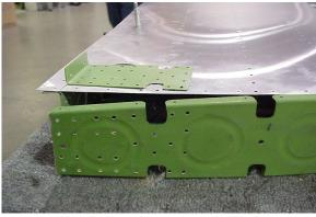
3/ Trim steel doubler provided to fit on the inside of rib. Trim back an eighth of an inch from the radius of the rib flanges and cut out slots for the stringers.
